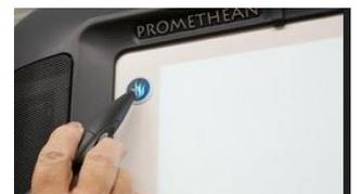
**RED:** Activboard has had trouble booting up or is not connected to a computer. Make sure the usb cable is plugged in tightly. Turn board off and then on again. Flame should turn white.
