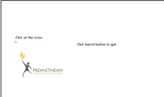
**Connect the ActivBoard before starting the computer.** When both the computer and ActivBoard are running, hold the ActivPen lightly on the ActivBoard without pushing in the nib; the cursor on the ActivBoard should line up with the ActivPen's tip. If it doesn't, the ActivBoard will need to be calibrated.
